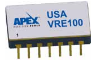
Hermetic 14-pin Ceramic DIP Package Style HC
